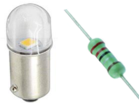
Optional: 1 or 2 BA9S LED Bulbs 180Ω 0.5W resistor (for 6V circuits) or 330Ω 1W resistor (for 12V circuits)
